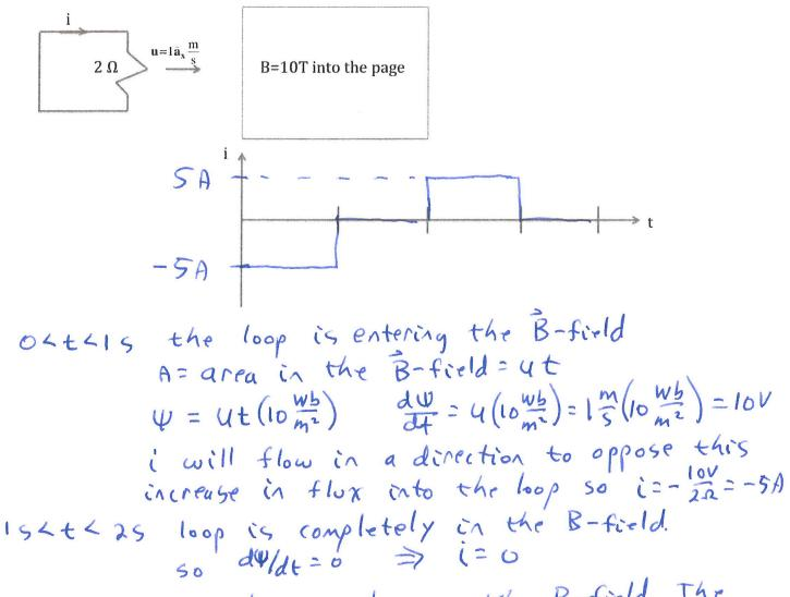
254 £435 the loop is leaving the B-field. The flux into the loop will now decrease at the same rate it was increasing for oxtx15 50 i= +5A
